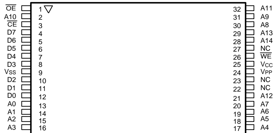
32-Pin TSOP — Reverse Pinout
