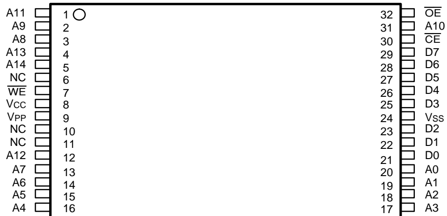
32-Pin TSOP — Standard Pinout
